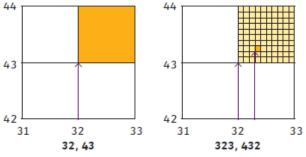
Four-figure and six-figure grid references.
