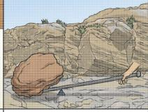
Levers can be used to make a small force lift a heavier load. A lever always rests on a pivot.
