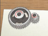
Gears or cogs can be used to change the speed, force or direction of a motion. When two gears are connected, they always turn in the opposite direction to each other.
